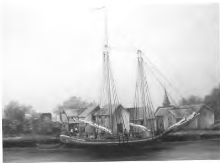
The James M. Carey was a two-mast schooner built in 1874. It had a length of 68.5 feet and a depth of twelve feet. (MHS)
