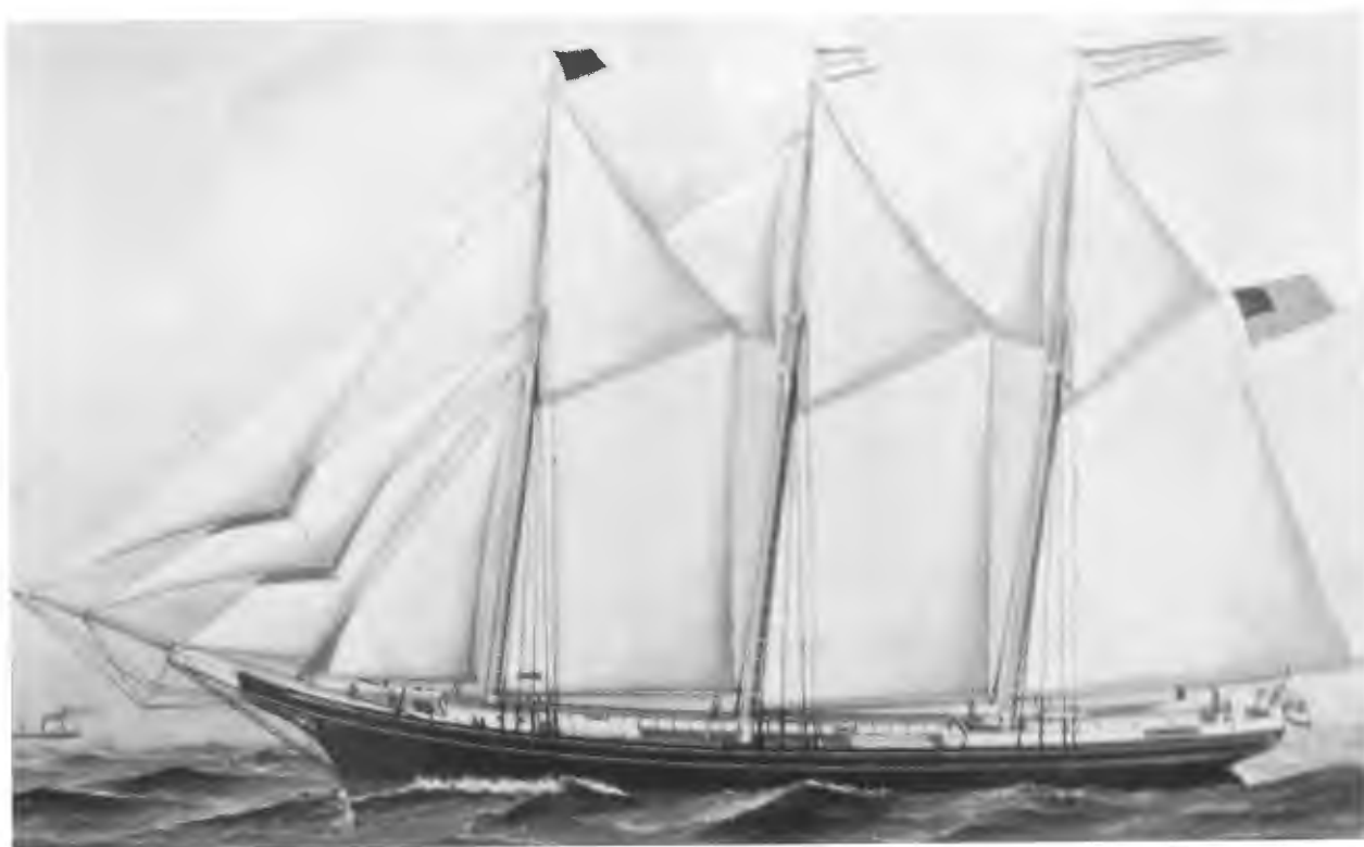
The Thomas Wismore was a three-mast schooner built in 1891 in Milton for Captain James Carey Conwell. It had a width of twenty-four feet, a length of almost seventy-nine feet, and a depth of six feet. (MHS)
