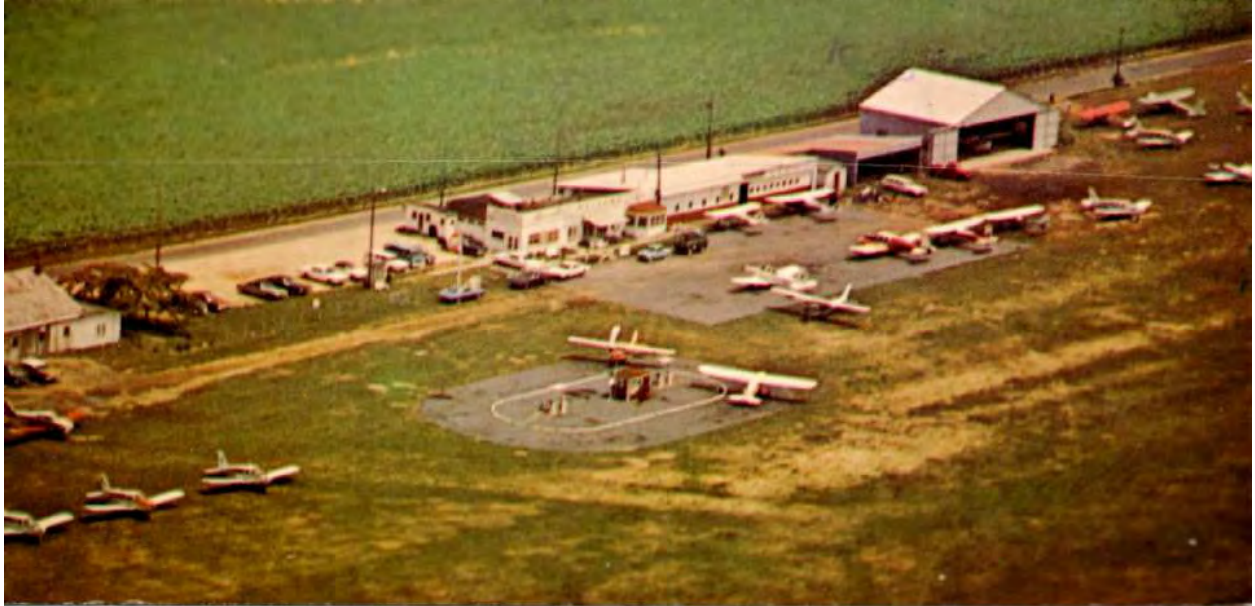
The 1975 aerial view looking northeast at Rehoboth Airport (courtesy of Philip Kineyko) depicted several hangars, an office/terminal building with a paved ramp, and a small paved area around the fuel island.
