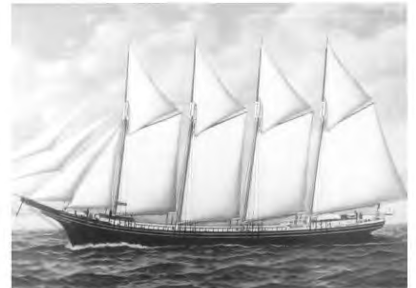
The Florence Creadick was a four-mast schooner built in Milton in 1890. She had a length of 164 feet, a depth of thirteen feet, and a width of thirty-six feet. She was torpedoed in July of 1915 off the coast of France and ended her career under the French flag. (MHS)
