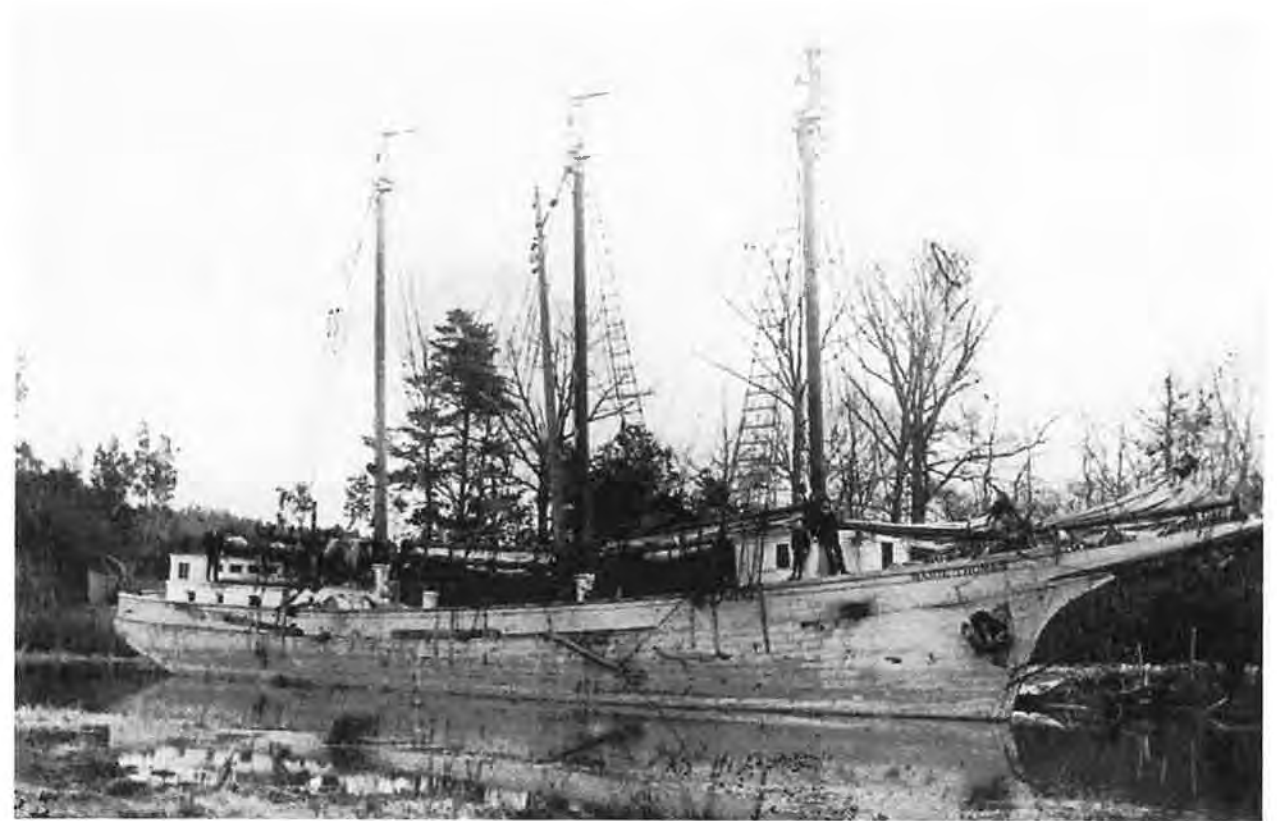
The Marie Thomas was the last local vessel built for local trading. Built in 1904 by James P. Davidson for Captain George E. Megee, it was a three-mast schooner and had an internal combustion engine. It was ninety feet long, about twenty-four feet in width, and had a depth of six and one-half feet. The Marie Thomas burned while docked at the Milton wharf in December of 1910. (Courtesy of Herman F. and Emily C. Black)
