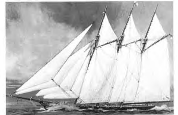
The Fannie Kimmey was a three-mast schooner, built in 1879. It had a width of almost thirty-three feet, a length of 129 feet, and a depth of twelve feet. (Courtesy of Herman F. and Emily C. Black)
