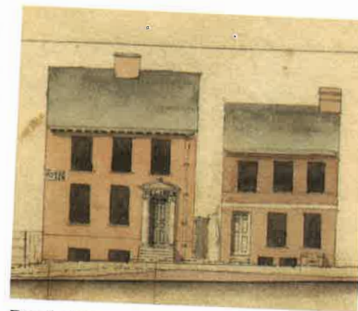
Detail of the Latrobe Survey's "Section of Front Street" shows how the street level would change for 6 and 8 The Strand, which explains their needs for front steps today. (Courtesy of Delaware Public Archives)
