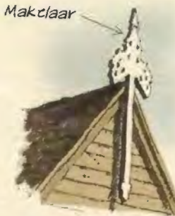
The curious ornamental features that can clearly be seen on the Lindeström elevation are most likely traditional Dutch gable ornaments called "makelaar."
