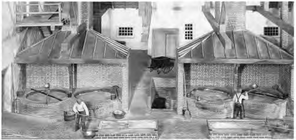
3.—PART OF A DIORAMA OF POWDER MAKING IN THE EXHIBIT BUILDING. This shows the refining of saltpetre in progress
